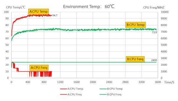
1. The following table shows the average temperature of the Raspberry Pi CM5 CPU during stable operation of the two groups of devices
