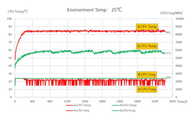
1. The following table shows the average temperature of the Raspberry Pi CM5 CPU during stable operation of the two groups of devices
